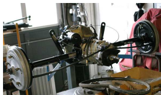
Restored transaxle ready to be installed.
